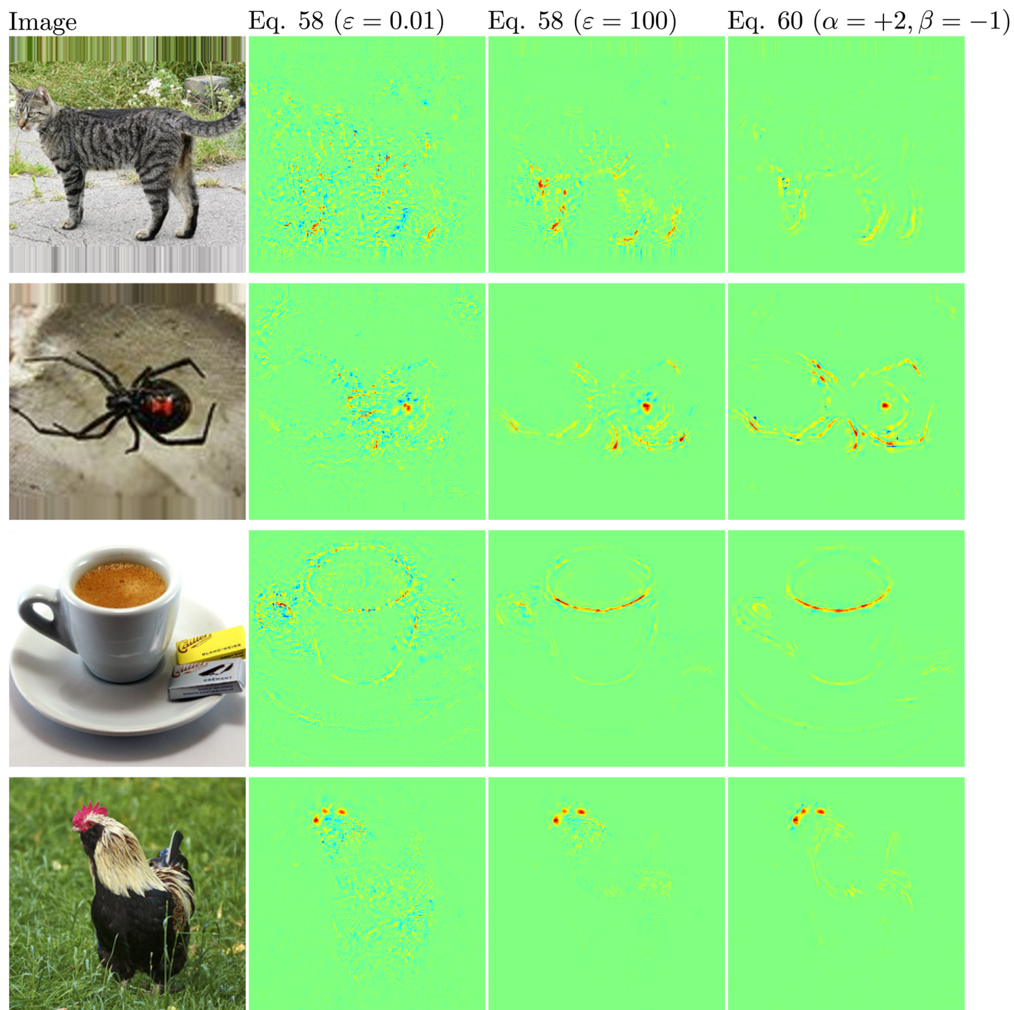
Fig 25. The pixel-wise decompositions for examples images of the neural net pre-trained on ILSVRC data set images and provided by the Caffe open source package [60]. Second column shows decompositions computed by Formula (58) with stabilizers \varepsilon = 0.01 , the third column with stabilizers \varepsilon = 100 , the fourth column was computed by Formula (60) using \alpha = +2, \beta = -1 . The artifacts at the edges of the images are caused by filling the image with locally constant values which comes from the requirement to input square sub-parts of images into the neural net. Pictures in order of appearance from Wikimedia Commons by authors Jens Nietschmann, Shenrich91, Sandstein, Jörg Hempel.
